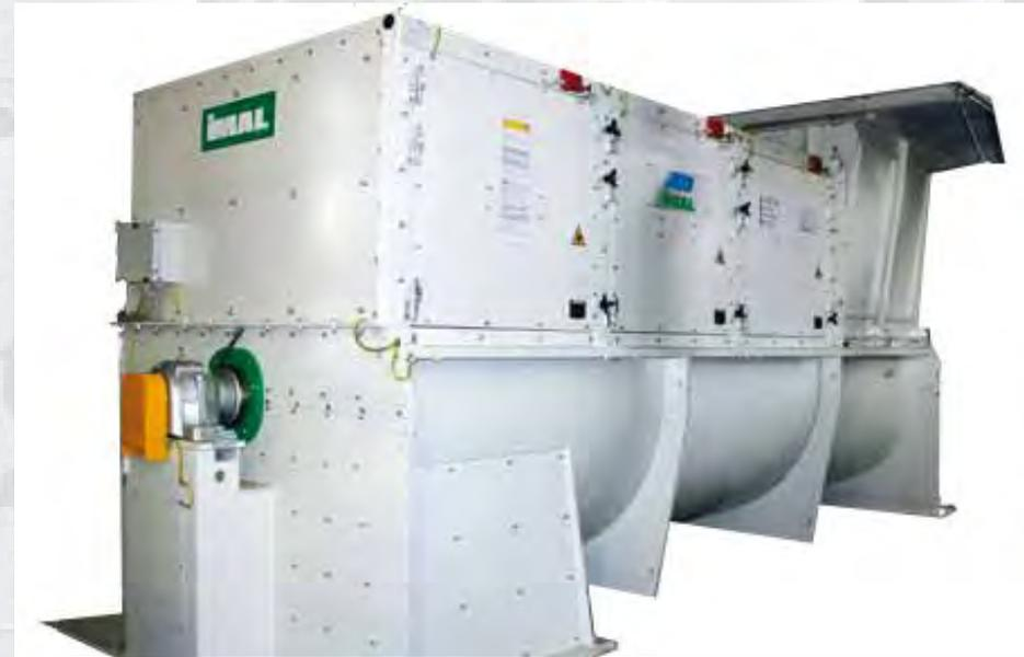
The special cooled chute is equipped with a motorized self-cleaning system, manifolds and mounts for the sprayer nozzles, and is used to convey the resined material to blender infeed.
